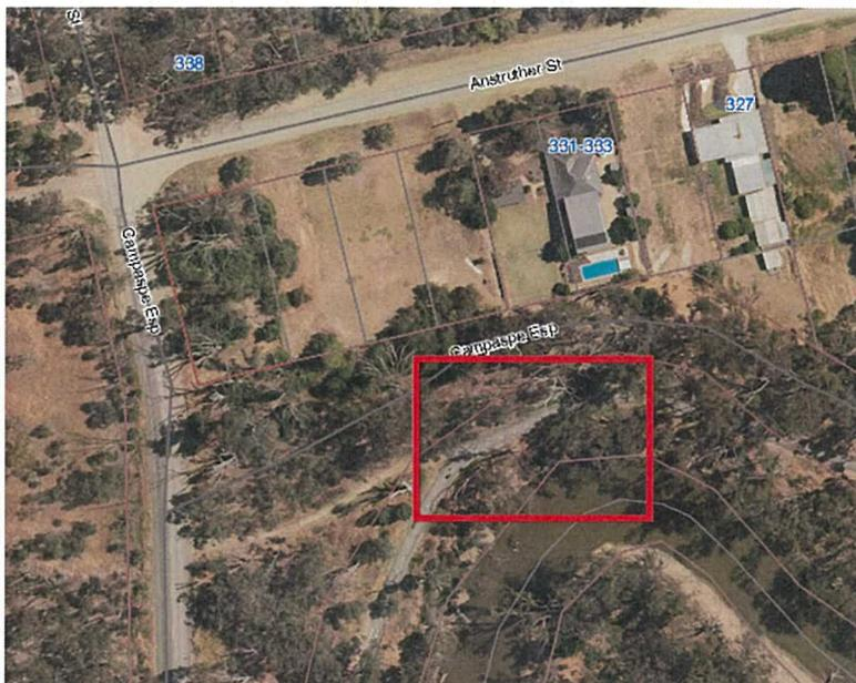
Significant erosion has occurred in this area and is now within 300mm of the edge of the path and is considered a hazard to users of the path. Further erosion threatens the integrity of the shared path and the safety of path users.
